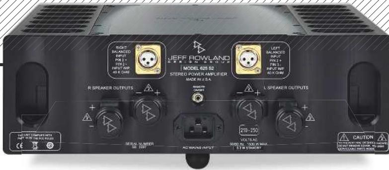
**ABOVE:** Balanced (transformer-coupled) inputs only, via XLRs, are joined by a pair of substantial screw-down cable connectors per channel. These are best suited to bare wire rather than 4mm or spade terminated loudspeaker cables
